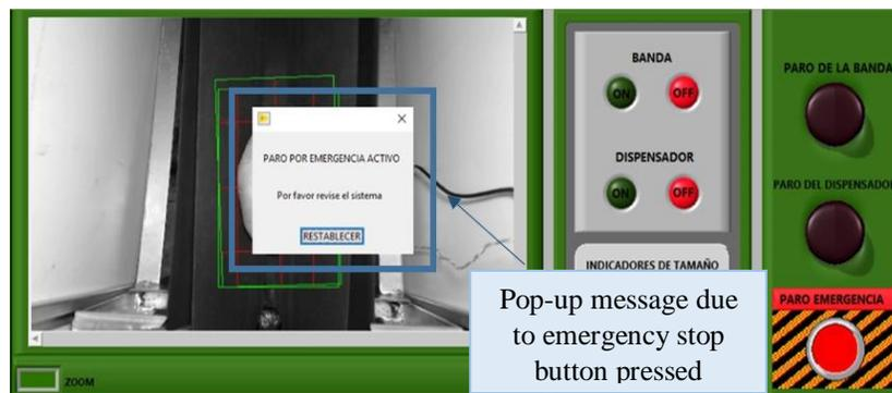
Fig. 9. HMI screen with emergency stop pop-up message.
