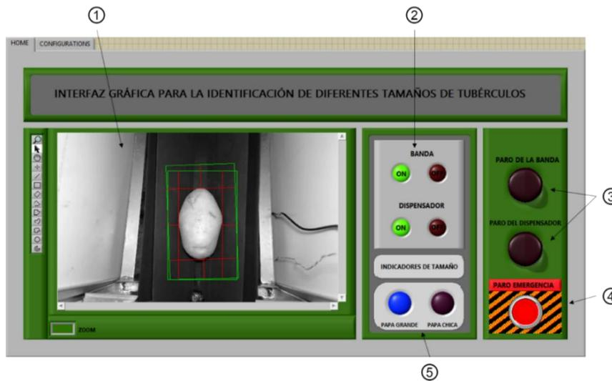
Fig. 8. HMI screen of the potato inspection and grading system.
