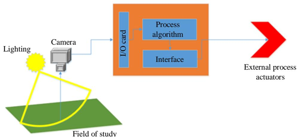
Fig. 1. Basic diagram of an image processing system.
