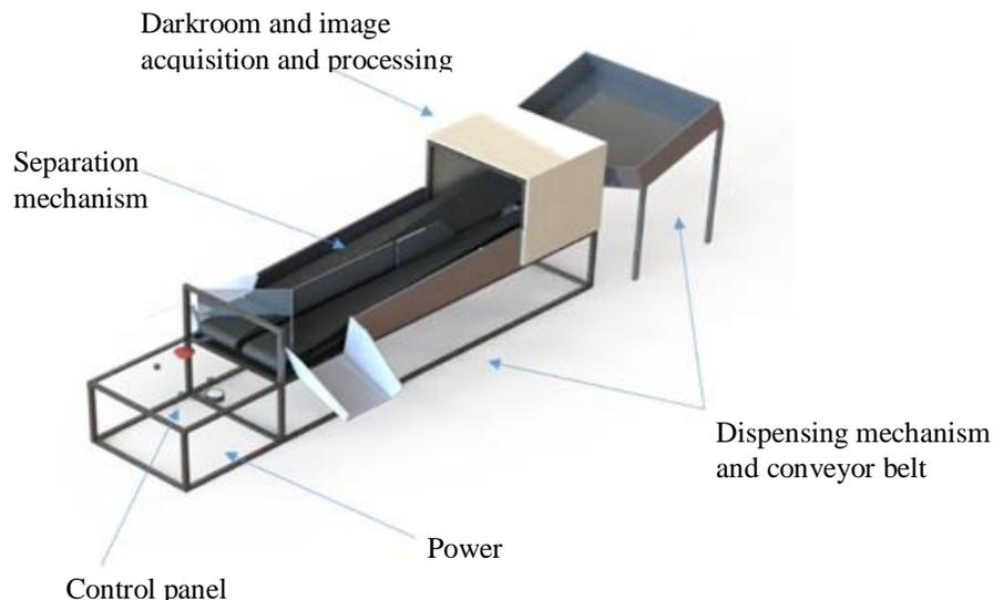
Fig. 3. Potato inspection and grading system scheme.
