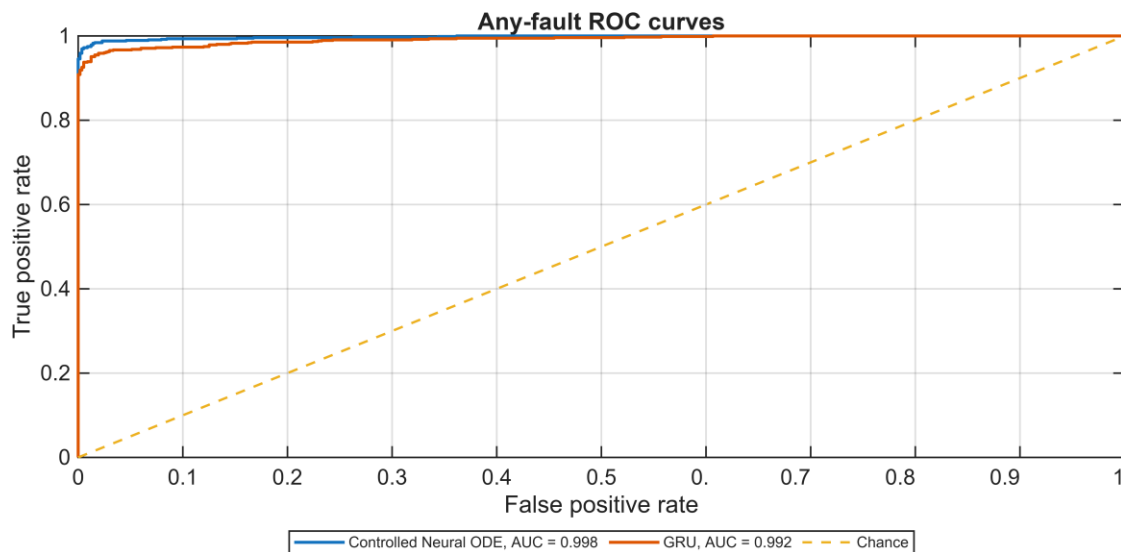
Fig. 11. Any-fault ROC curves obtained by aggregating battery, motor, and overheating faults into a single nonhealthy class.
