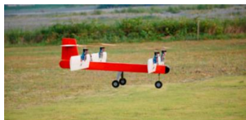
(e) Quad Tilt Wing (QTW) VTOL [19].
